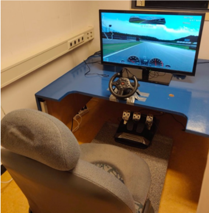
Figure 1 The set-up of the driving simulator used in both the experimental driving and passive viewing control conditions. It consisted of a chair, steering wheel, pedals and a 23-inch flat screen. A PlayStation 3 and the game Gran Turismo (Yamauchi, 2013) were used to simulate the actual driving experience. Participants drove (or viewed a recorded video of) three laps on the Twin Motegi Course.
